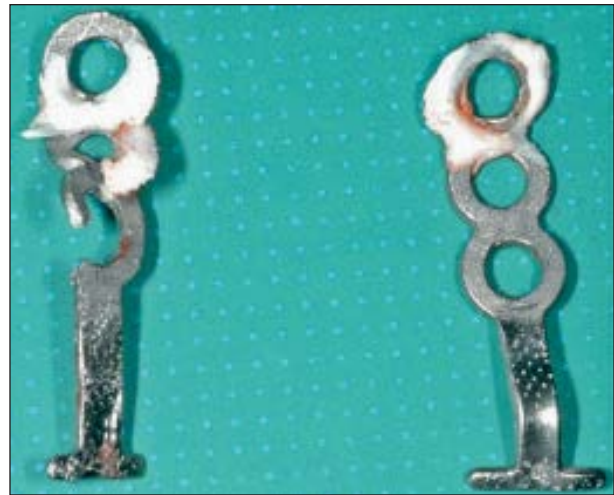
Fig 5 Bone overgrowth is clearly visible on the fixation plate of the OBA. In this case, removal of the miniplate was difficult, which explains the breakage of the plate through torsional force and the imprints of a removal instrument on the OBA.
